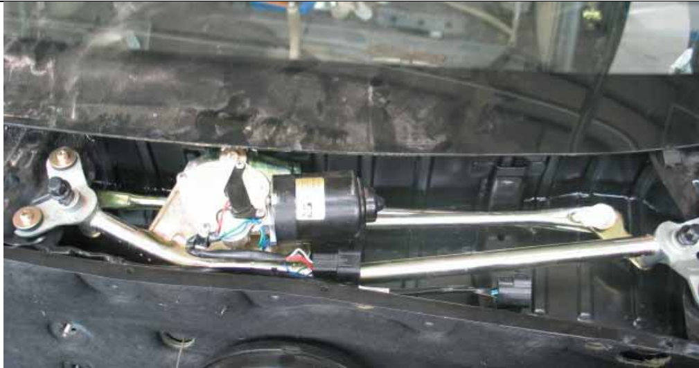
Installation of the wiper abutment
