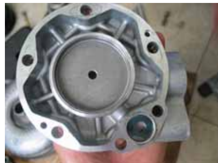
Inside structure of the compressor3
