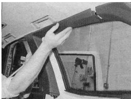
26.30 ... free the door pillar trim panel from the sealing strip, and remove it from the vehicle
