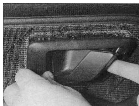
12.2 Lift the door inner handle, and remove the escutcheon from the door
