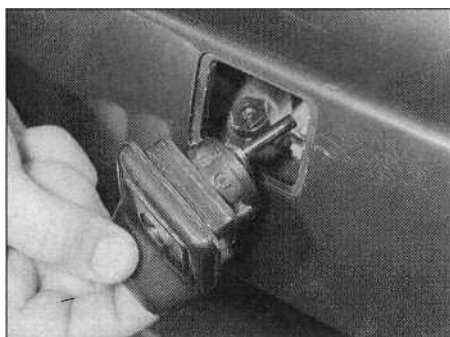
16.3b ... then withdraw the lock cylinder and handle assembly from the tailgate
