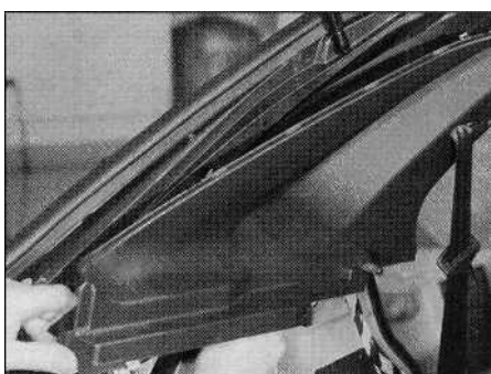
26.20c ... and free the upper trim panel from the luggage compartment - five-door model shown
