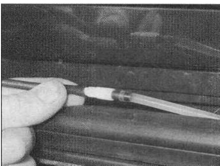
15.4 Release the tailgate washer pipe from underneath the sealing strip, and disconnect it at its non-return valve
