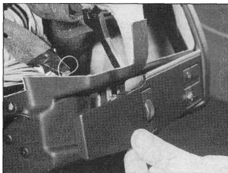
28.7b ... and right-hand switch panel, and remove them from the fascia (right-hand-drive model shown)
