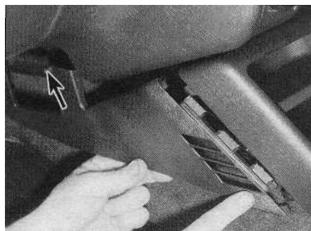
27.2 Removing the centre console left-hand front side panel - retaining screw location arrowed
