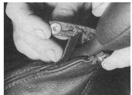
27.3a On models with a leather gear lever gaiter, release the pop fastener and velcro strip...
